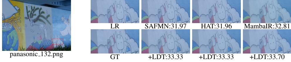
Figure 4: Visual comparison of LDT. The large image on the left is the LR image, and the sub-images on the right are LR, SAFMN, HAT, MambaIR (first row), GT, SAFMN + LDT, HAT + LDT, MambaIR + LDT (second row). The value following the name represents the PSNR metric of the current patch.
